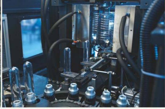
SMLA series is specially designed for extra large bottle production with volume between 5L to 10L, and the output is from 12008PH to 2500BPH per unit.
