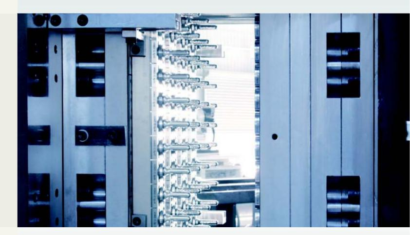
PET Preform Injection Molding Machine PET瓶胚注塑机
